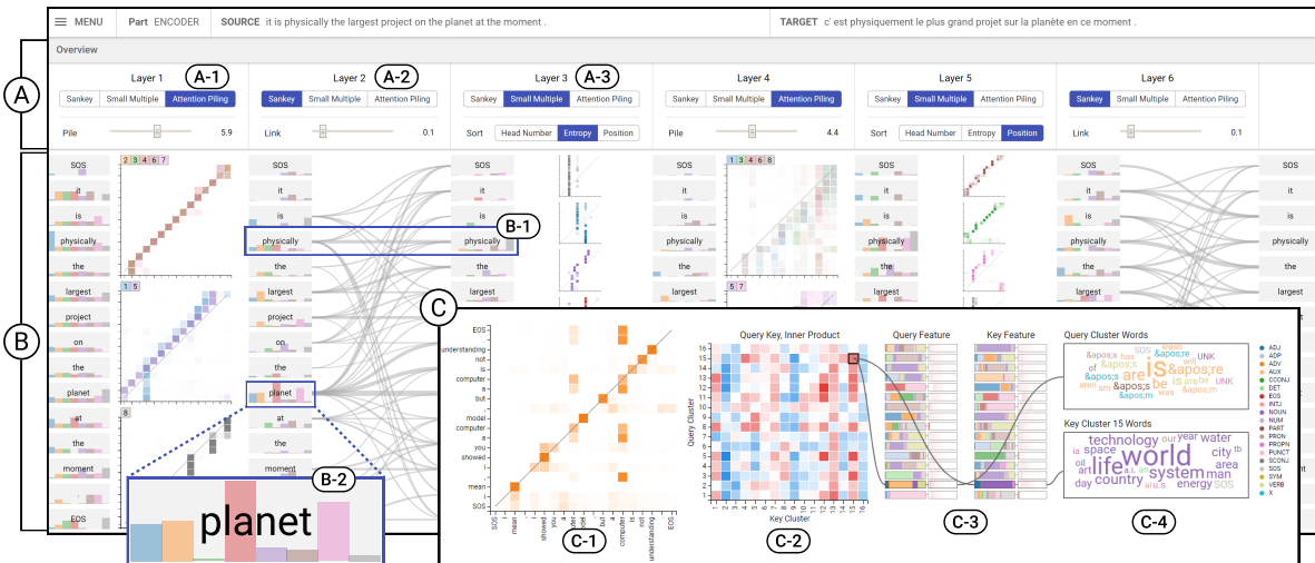
Figure 1: Overview of SANVis. (A) The control panel presents three types of visualization options: (A-1) the attention piling view, (A-2) the Sankey view, and (A-3) the small multiples view. (B) The network view displays multiple attentions for each layer according to a selected visualization option. (B-2) Different color bar heights indicate the average attention weights based on different heads (eight heads in total) at each layer. (C) The HeadLens helps the user analyze what the attention head learned by showing representative words and by providing statistical information of part-of-speech tags and positions.
