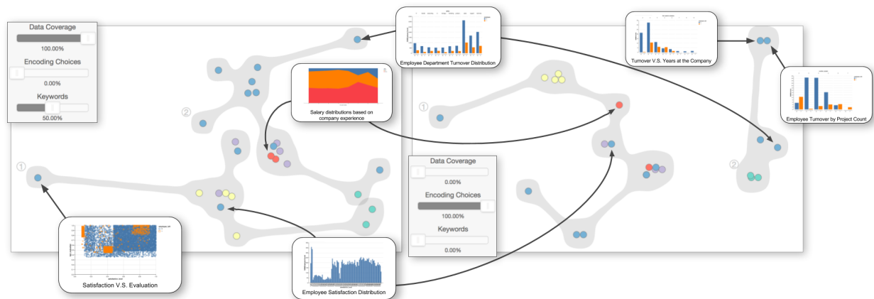
Figure 1: An analyst is using Constellations to investigate results generated by previous analysts. Constellations organizes these visualizations with projection and clustering. Adjusting the data coverage, encoding choice, and keywords sliders changes how pairwise chart similarities are scored and updates the projected layout and cluster groupings. Several charts are tagged to show how their positions change.
